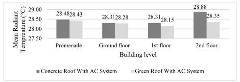
Figure 1: Comparison of simulation results for average MRT temperature for 4 levels of study building on 29 March 2022 from 6.30 to 18.30. Source: Authors (2022).
