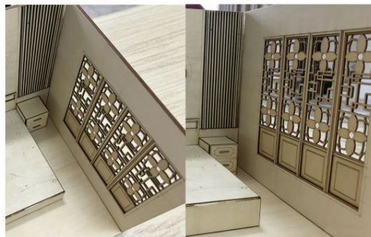
Figure 7: Model-scale lingzhi-based screen prototype showing modular repetition, wall integration, and visual permeability
