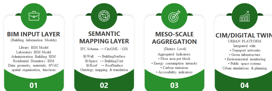
Figure 7: Workflow illustrating the application of the BIM-to-CIM Integration Framework (BCIF) within a university campus district. The diagram shows the transition from building-level BIM models to district-level CIM analytics through semantic mapping and meso-scale aggregation.
