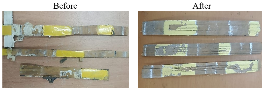
Figure 3.0: Before and After ASTM D3039 Testing
